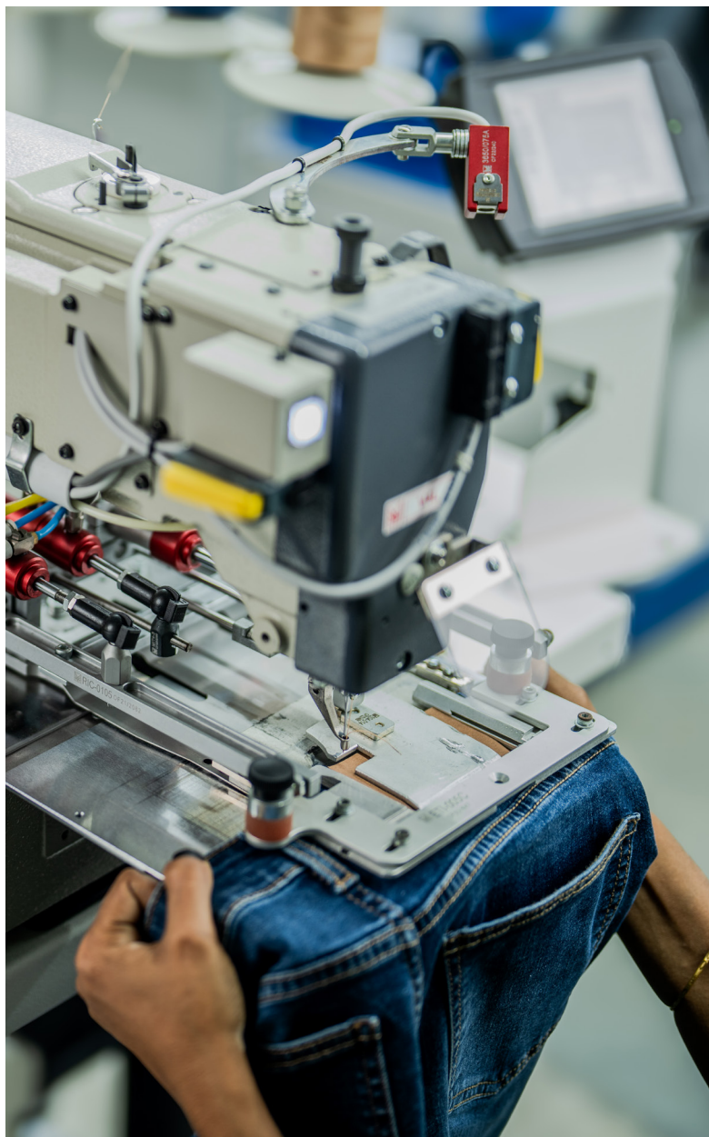
LEATHER PATCH ATTACHMENT MACHINE
